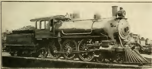
4-6-2 Type Simplified and as Used on Plant System
